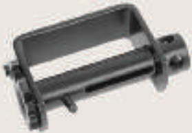
41681-10 Standard Bottom Mount Weight: 10.6 lbs./4.8 kg. WLL: 5,500 lbs./2,500 kg.
