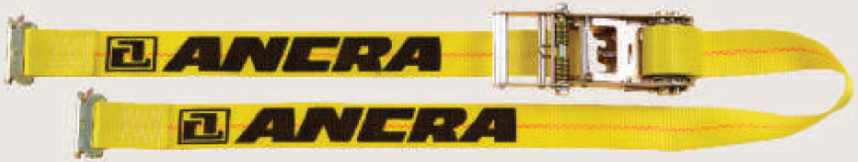
Series E Heavy-Duty Buckle Strap w/ Spring E Fitting Heavy-duty 12,000 lbs. yellow latex treated polyester webbing. WLL: 1,333 lbs./605 kg. Fixed End: 48-in.
